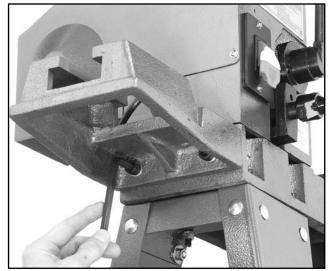
Figure 11. Attaching extension table.
